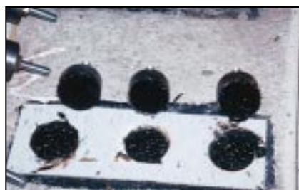
Figure 3. Pull-off tests usually resulted in cohesive failures within the tile adhesive.
