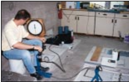
Figure 2. Using a manually operated screw piston, a technician applies pressure from a hydraulic ram to pull off vinyl-composition-tile plugs.
